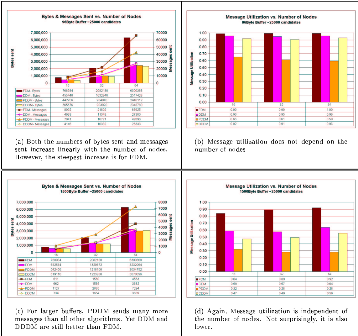
Figure 6: Message utilization (5 and 5) remains stable regardless of the number of nodes. Hence, since our algorithms are scalable with respect to the number of bytes sent, they are also scalable with respect to the number of messages sent. However, this scalability does not suffice in the case of PDDM and large buffers because the initial number of messages is so much larger than that required by FDM that it remains the largest even for 64 nodes. DDM and DDDM, on the other hand, are better in both respects than FDM.
