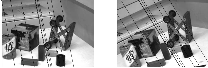
Figure 2: Two images of a scene. Ten pairs of corresponding points have been extracted and the points (denoted by the circles) and their respective epipolar lines have been overlaid over the original images.
