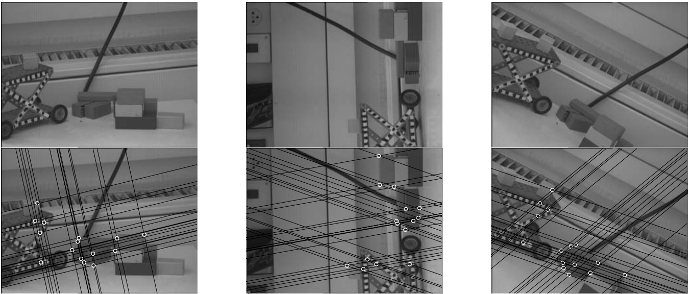
Figure 9: Top: three images of a scene. Bottom: 15 triplets of corresponding points have been extracted and the points (denoted by the circles) and their respective epipolar lines have been overlaid over the original images.
