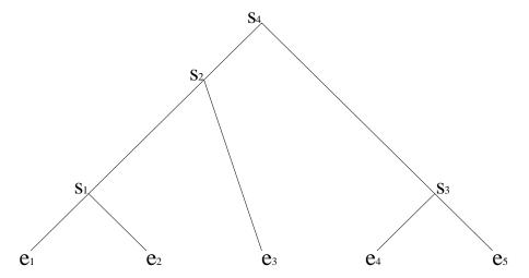
Figure 1: The global algorithm can be described as a binary tree where the leaves are the extrema and the inner nodes are the saddle points closest to the subsurfaces represented by their children.
