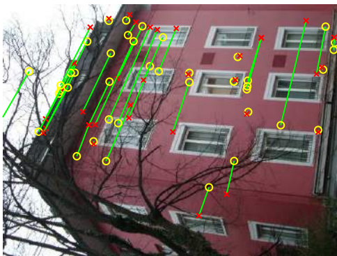
Fig. 9. Wrong matches of non-repeating keypoints that result from repetitive elements. Original image with non-repeating keypoints \mathbf{x}_i' marked by yellow circles and \mathbf{x}_i'' by red crosses. Green lines are proportional to the projective depth \rho_i .
