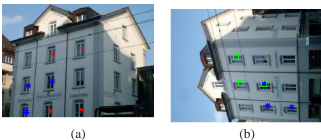
Fig. 5. Typical results, when building a list of all possible homographies. (a) Blue stars: An arbitrary point with its vertical and horizontal nearest neighbors within the same cluster. Red points: Additional points from the same cluster, that support the same H . (b) Blue stars: correct point match and its nearest neighbors. Green squares: An alternative point match.
