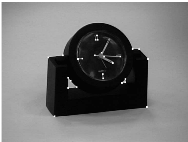
Fig. 6. Experiment setup. The image of the clock used in the experiment. The results of the corner detector which were the input to the algorithm are overlaid over the original image.
