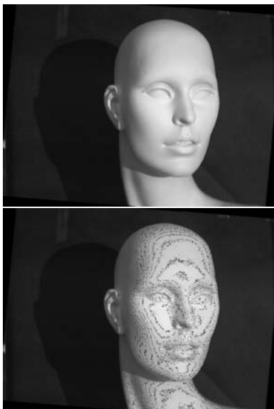
Fig. 3. Mono-geometric-stereo: (a) A real image of a mannequin with non-frontal viewing position and frontal illumination; (b) Iso-intensity contours are overlaid over the image demonstrating the equal intensity for corresponding points. For images like this, a variant of a stereo algorithm can be applied.
