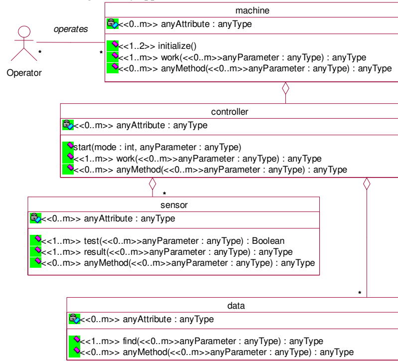
Figure 2. A UML class diagram describing a domain of sensor-based machines
