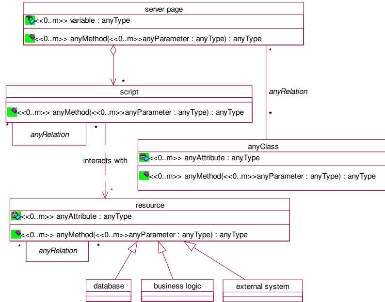
Figure 3. A partial class diagram of a Server Page in the Web application domain
