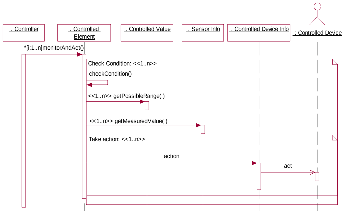
Figure 3. The PCS domain model in ADOM-UML: a sequence diagram of monitoring & acting.
