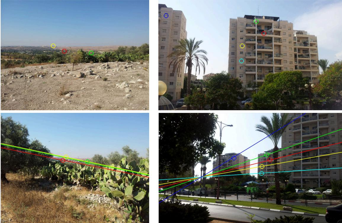
Figure 1: Wide baseline images for which the epipolar geometry could not be estimated using current algorithms but was successfully estimated by SOREPP. Left: *Open* set. Right: *Urban* set. Top: The reference image with several control points marked. Bottom: The target image after matching with the control points and their corresponding estimated epipolar lines.
